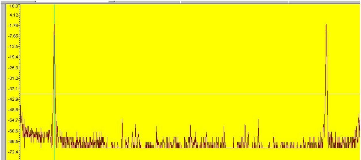
Figure 9 – ADC-A at 10.0MHz , Kaiser-Bessel window
