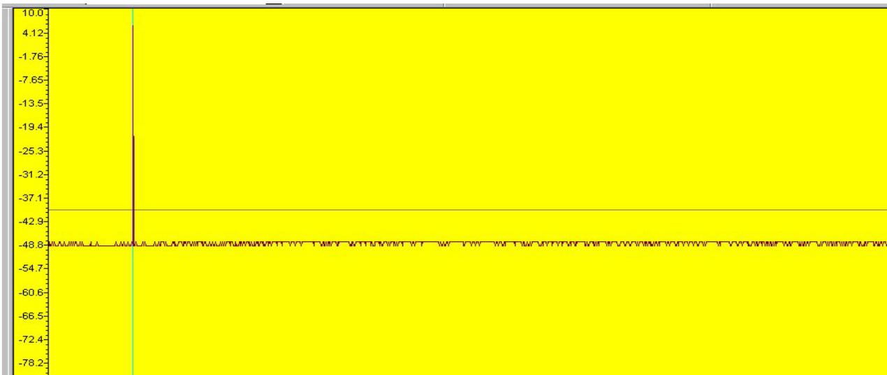
Figure 5 – DDS at 10.058MHz , Rectangular window
