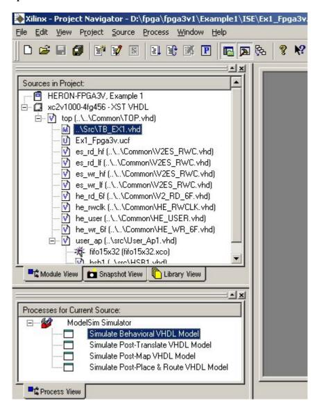
With the test-bench selected, double-click on 'Simulate Behavioral VHDL Model'. At this point ModelSim should start.
