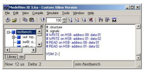
As we can see above, in this simulation two write accesses were made over the HSB message interface. The first access was to address 0 (to set the Input FIFO number used) and the second access was to address 1 (to set the Output FIFO number). These accesses were then followed by two read accesses to check the values that were written.
