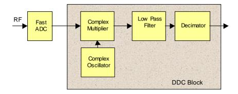
Figure 3 - A Theoretical DDC Block Diagram
