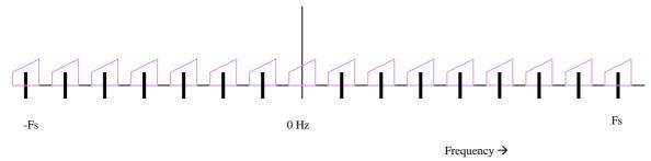
Figure 8 – Spectrum of quadrature signal after decimation Sample frequency Fs/7
