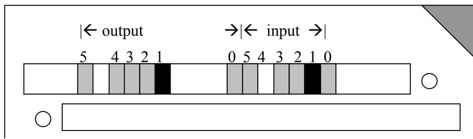
These jumpers are used to select the default routing of FIFO 0 on the Carrier card. This is to enable the actual source of the boot stream to be set up, even before the application starts and configures the system connectivity to be used.
