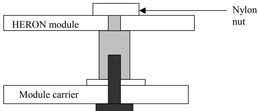
If the environment demands, the secondary fixing pillars can be fitted to modules that allow their use.
