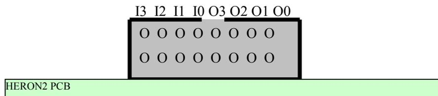
All pins on this side of the connector are connected to ground
