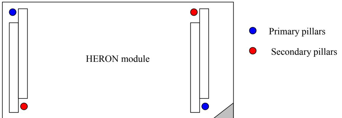
The Carrier card will probably only have spacing pillars fitted to the primary location for each HERON slot. The pillars for the secondary locations will be supplied as an accessory. The reason for this is that the legacy GDIO modules cannot be fitted if the secondary pillars are in place.
