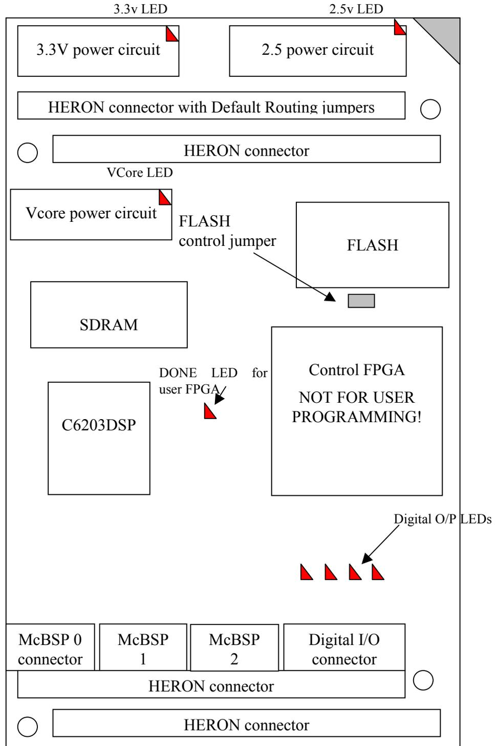
The HERON2 is a module that plugs into a HERON module carrier.
