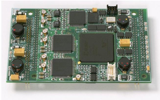
***HERON-IO5 FPGA module with 2 channels of 12bit 210Mhz A/D and 2 channels of 16bit 160Mhz D/A***
